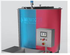
Double jacketing for cooling/ heating and insulation
