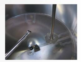
High speed crushing propeller
