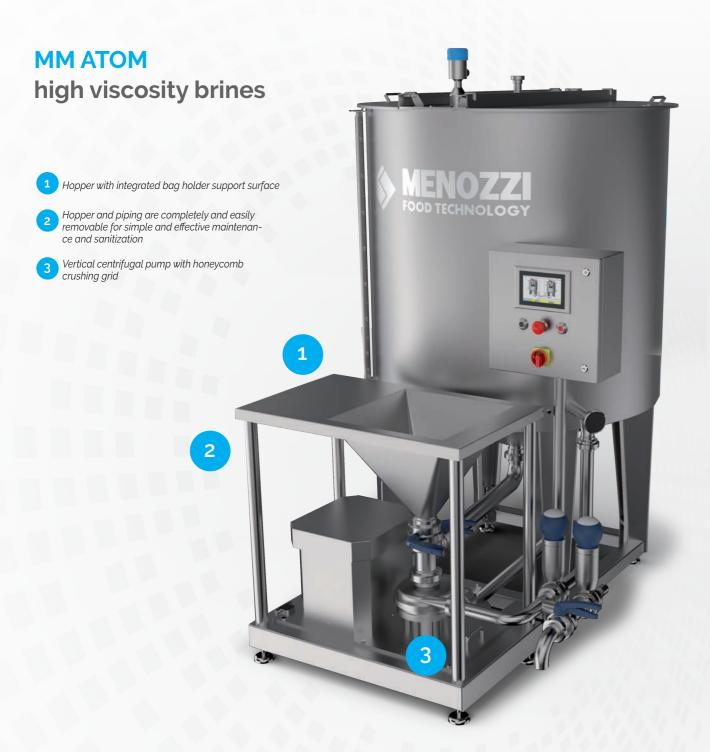
Menozzi High Shear Mixers MM-ATOM 1000-3000 are employed to produce viscous emulsions, that is to dissolve in water ingredients such as: starches, proteins, pectines, karrageen and caseinesinates or for the preparation of saturated brines.
