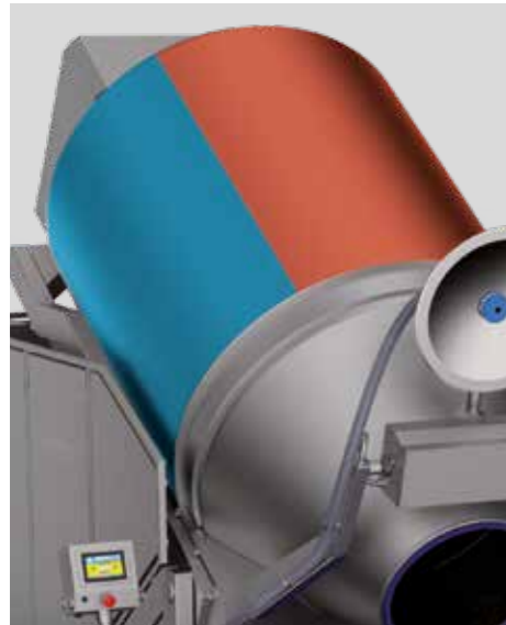
Refrigerated-heated jacketing with automatic thermal control
