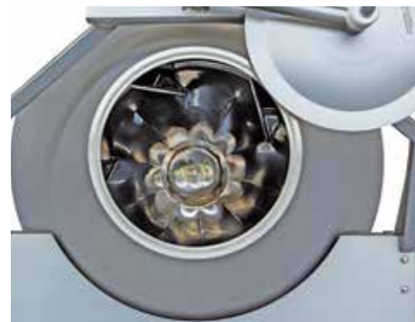
Mirror- polishing of the internal surface of the drum
